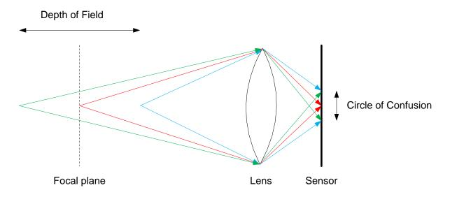
The diameter of the lens defines the aperture through where light is received, larger the aperture more light is received. This aperture is known as F/stop and can be controlled by a mechanical iris. It is a fraction of the lens diameter and is defined by a number F/i. So, f/2.8 allows nearly all light coming through the lens to reach the sensor, while f/16 allows a much smaller amount.
