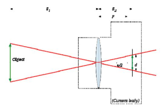
To project a sharp image of distant objects, S2 needs to be equal to the focal length, F or f, which is attained by setting the lens for infinity focus. Then the angle of view is given by:
